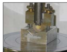
Figure 2. Shear Bond Test Set-Up
